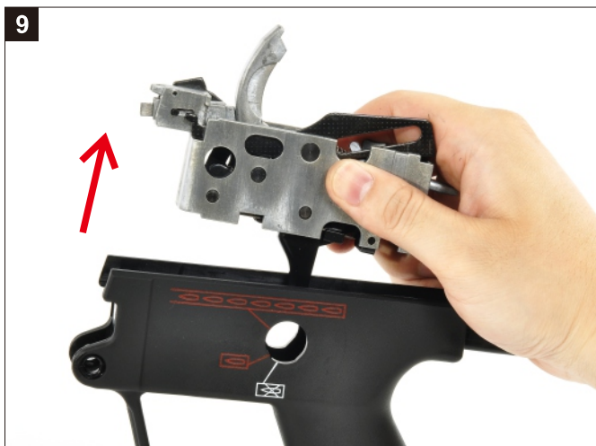
移除扳機組，完成。 Pull the Trigger Mechanism out of the Plastic Grip.
