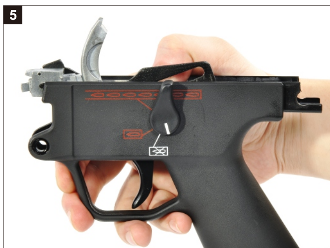
承上，將選擇鈕撥桿旋轉如圖。 Looking at the left side of the Trigger Group, rotate the Selector Lever in a clockwise turn until it stop with the white indicator line pointing down.
