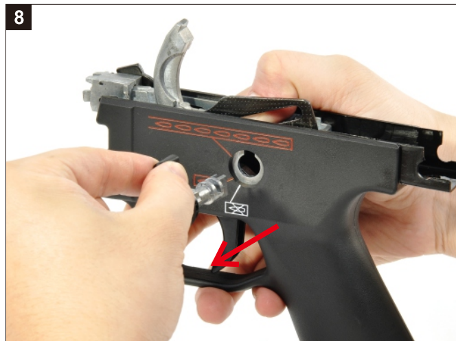
移除左側選擇鈕撥桿。 Remove the Selector out of the left side of the Trigger Group.
