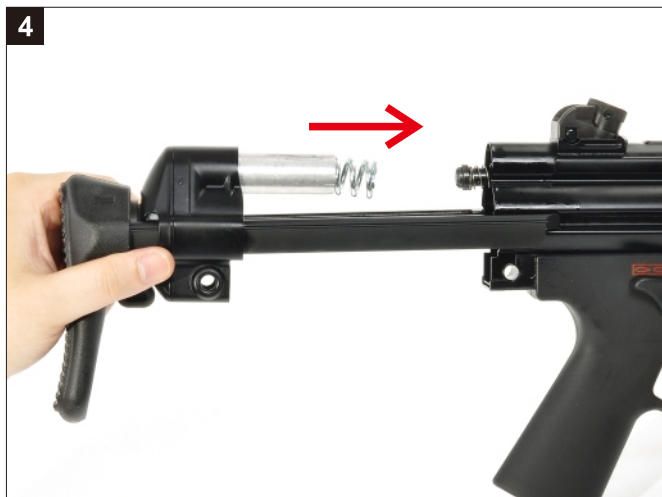
注意相對位置。 Make sure the retractable stock is in the right position.
