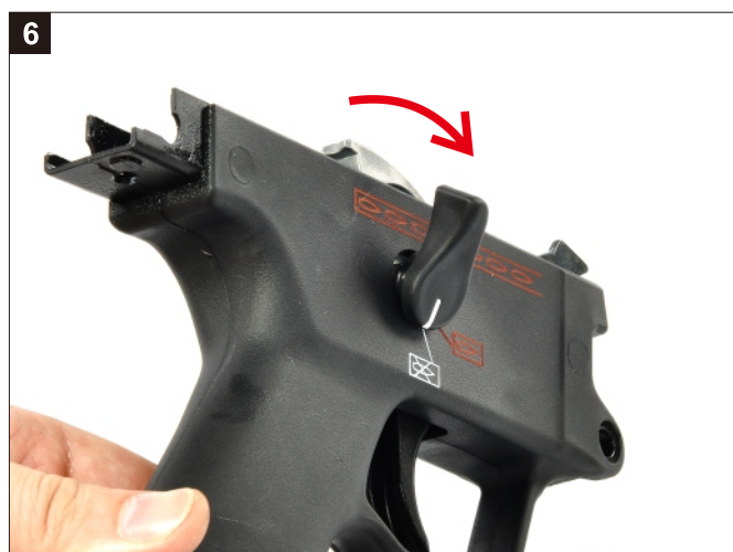
移除右側選擇鈕撥桿。 Remove the Selector Lever from the right side of the Trigger Group.
