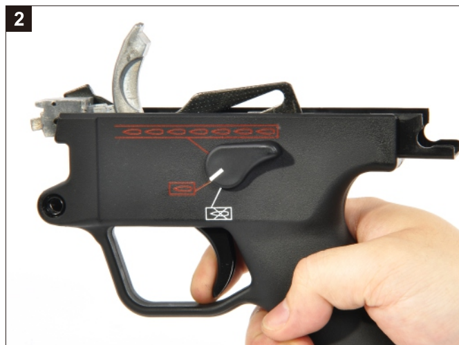
扣壓扳機釋放擊錘。 Pull the Trigger and allow the hammer to snap forward.
