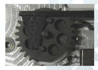
As such, tappet plate modification is necessary. Simply measure and mark off a distance of 11mm from the base of the tappet plate. Then snip off the excess portion as shown below.
