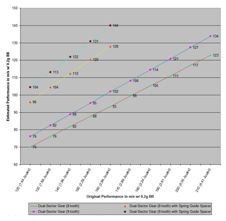
Actual performance may vary due to the variety of components used. In a Cyclone Dual-Sector Gear System without the spring guide spacer, the spring can produce anywhere from 30% to 50% of the energy producible in a traditional full stroke setup. When the spring guide spacer is used, 60% to 70% of the spring's energy can be achieved. *Please also note that the original performance figures listed are actual spring performance and are not indicative of the manufacturers' spring ratings*.
